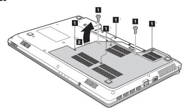
**6** Remove the frame fixing screws **3**.
